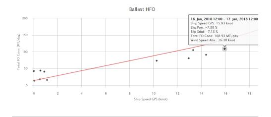
The above figure shows the actual vessel performance, shown as daily "dots", relative to the contractual conditions, indicated by the red line.
